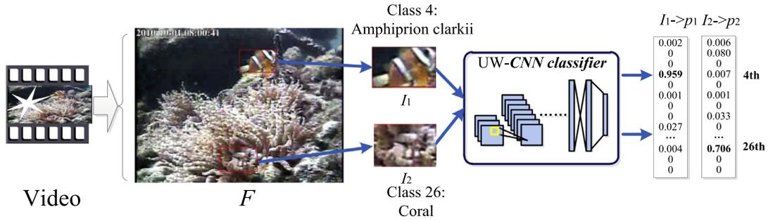
Fig. 3. An illustration of the object classification procedure for one frame.
