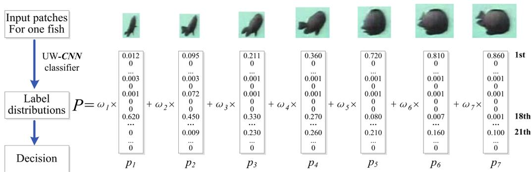
Fig. 4. An illustration of the trajectory based fish recognition.
