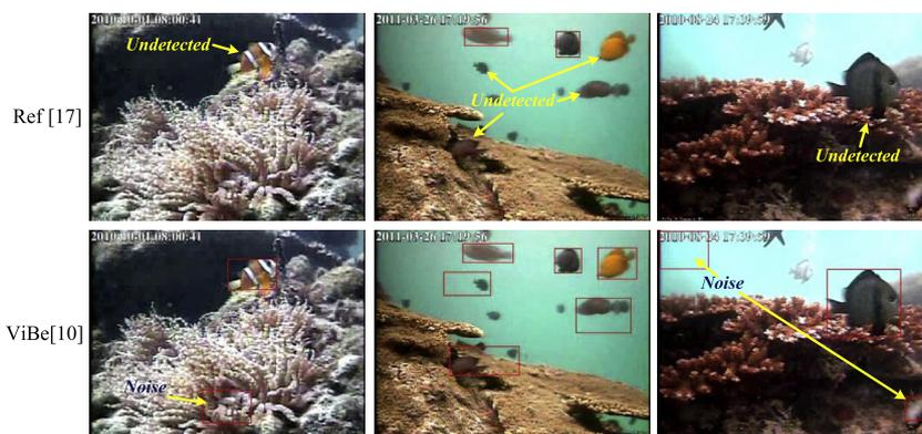
Fig. 6. Results of two different fish detection methods.
